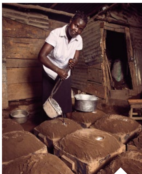
Businesswoman pours molten metal into dirt-covered moulds to make 120-230 cooking pots each day, Kampala, Uganda.
